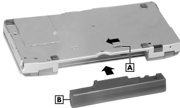
**A** – Battery release lock **B** – Lithium-Ion battery pack
