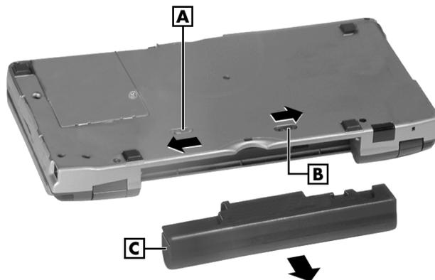
**A** – Battery release latch **B** – Battery release lock **C** – Battery pack
