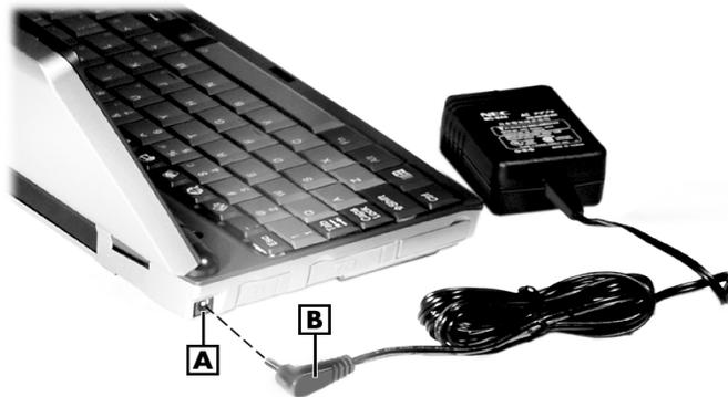
**A** – AC Power port   **B** – AC adapter cable
