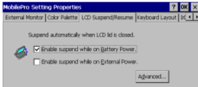
3. Select either “Enable suspend while on battery power” or “Enable suspend while on external power,” or both, to enable the display linkage switch.
