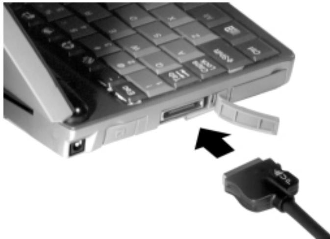
3. Connect the other end of the cable to the 9-pin serial port on your host PC. If your host PC has a 25-pin serial port, use an adapter (available in most computer stores).
